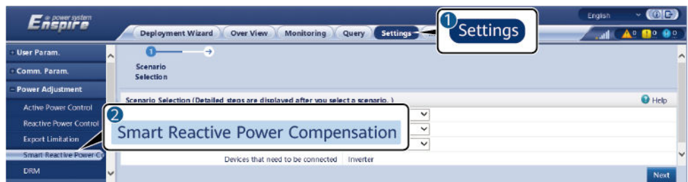
Figure 6-87 Setting parameters for smart reactive power compensation (Scenario Selection)
