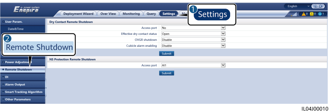
Figure 6-94 NS protection remote shutdown
