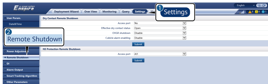
Figure 6-92 Dry contact remote shutdown
