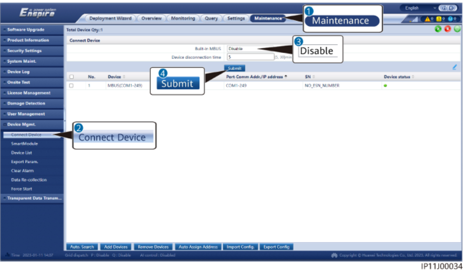
Figure 6-54 Setting parameters for a built-in MBUS module
